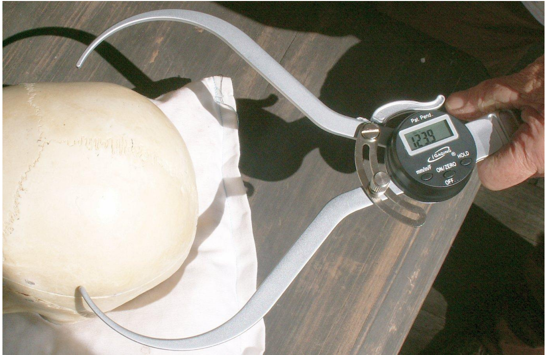
Figure 4. Digital spreading calipers.
