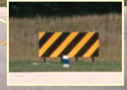
The purpose of the taxiway ending marker is to prevent pilots from taxiing off the end of the pavement at locations where pilots are not expecting the taxiway to end.
