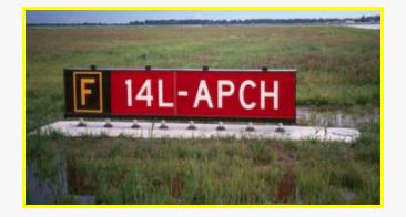
At some airports it may be necessary to hold aircraft on taxiways located in the approach or departure corridor of the runway so that the taxiing aircraft does not interfere with the operations on that runway.
