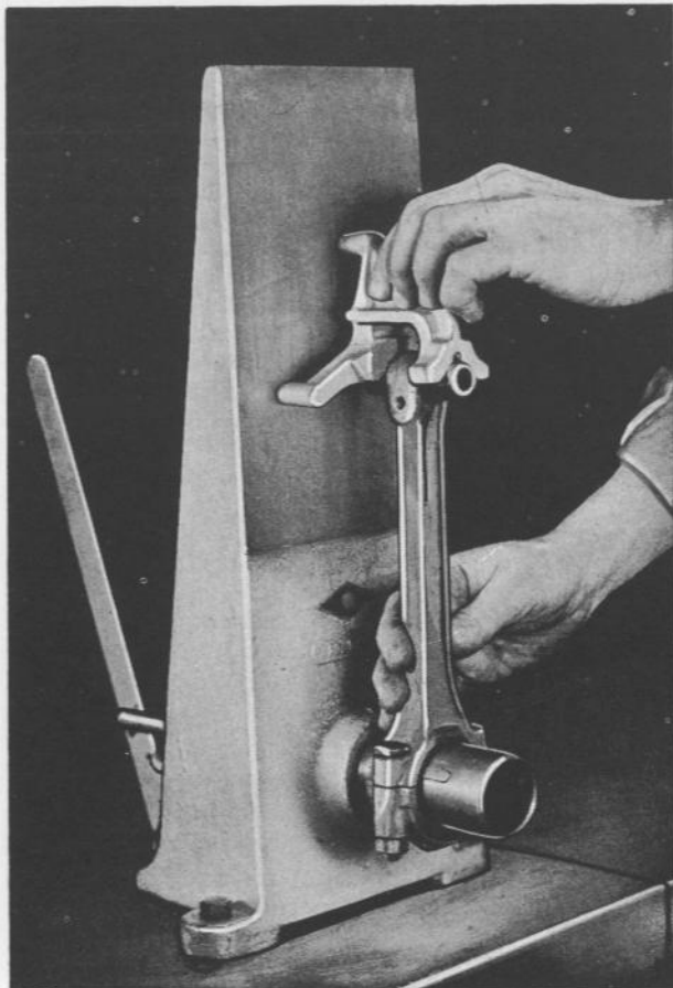
FIG. 29—CONNECTING ROD ALIGNER
