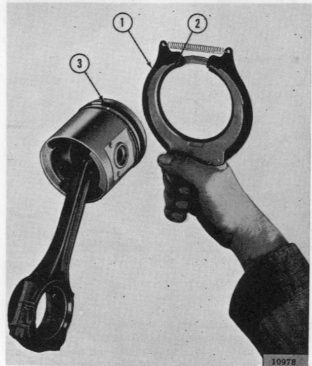
FIG. 95—INSTALLING RINGS ON PISTON
