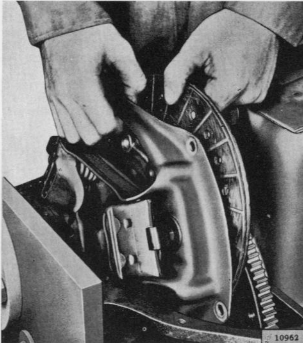
FIG. 79—REMOVING CLUTCH ASSEMBLY FROM CLUTCH HOUSING
