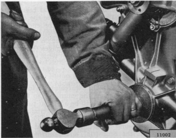
FIG. 131—INSTALLING FRONT CRANKSHAFT OIL SEAL WITH TOOL W-269
