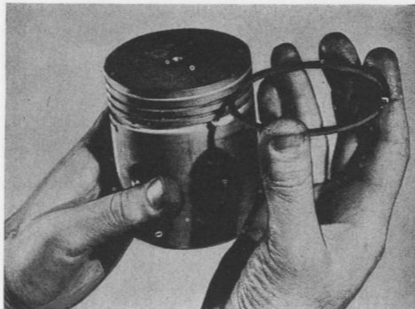
FIG. 35—COMPRESSION RING FITTING
