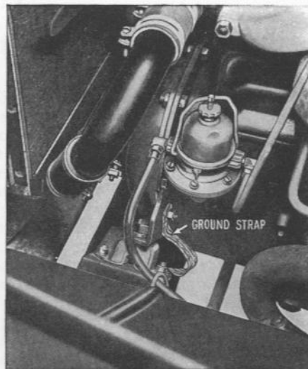
FIG. 46—ENGINE GROUND STRAP
