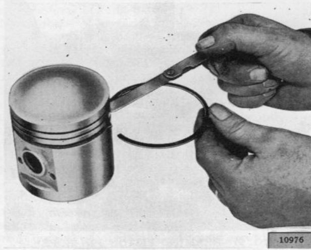
FIG. 93—CHECKING PISTON RING SIDE CLEARANCE
