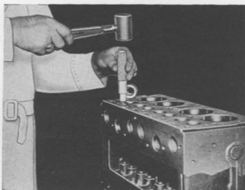
FIG. 12—VALVE GUIDE DRIVER
